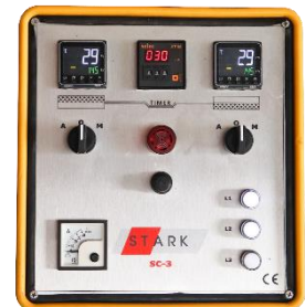
Electronic control box with data logger for regulating temperature
