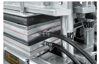
Rubber pressure bag for even distribution
